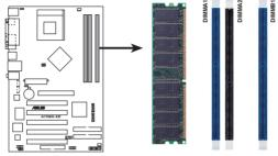
A7N8X-XE 184-pin DDR DIMM sockets
